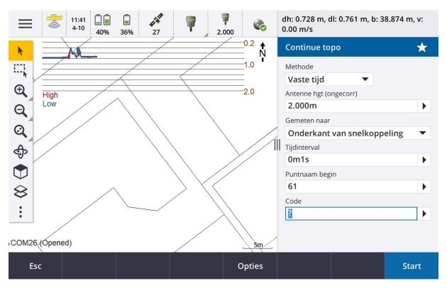
The depth graph also shows the high frequency (red) and low frequency (blue). When a single frequency echosounder is being used, the graph will show only a red profile.
