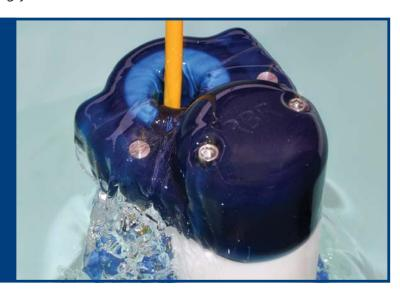
The MLM-1000 consists of two major components; the head end modem (HEM) and the sub surface modem (SSM). Each instrument on the mooring line system is connected to an SSM which communicate with the HEM (and host) through the mooring cable inductively.
